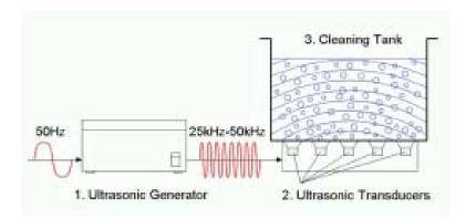
Figure 1 Sonic Cleaner Unit Diagram
