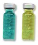
Figure 5 and 6 SonoCheck<sup>TM</sup> Results Yellow= Positive Change/Effective Cavitation Blue/Green=No Change/Ineffective Cavitation
